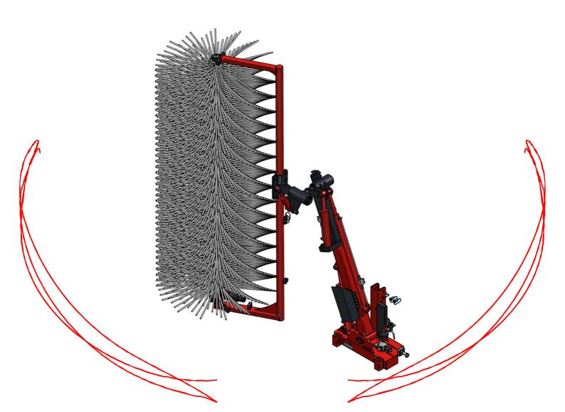
Fruit thinning machine for orchard, mounted on a front II category lifter with electro-hydraulic controls via joystick.
